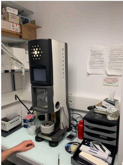
Figure 3. Vitrobot plunge freezer
