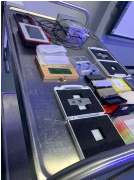
Figure 2. Collection of numerous testing tools for quality control and standardization in light microscopy.
