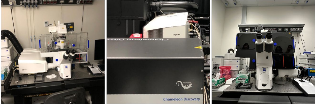
Fig4. Light microscopes at Human Technopole. Left: Confocal microscope LSM980, middle: Two-photon microscope system, right: Structural Illumination Microscope.
