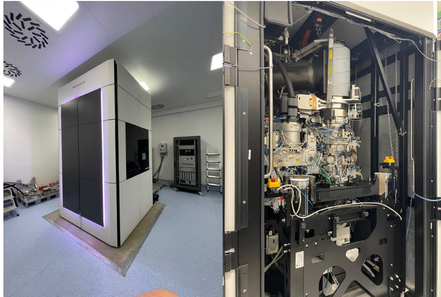
Fig3. Two electron microscopes at Human Technopole. Left: Spectra 300kV STEM, Right: Titan Krios G4i 300kV TEM
